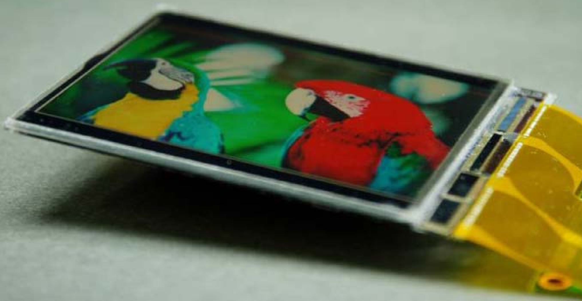
Most recent reflective color LCD (Test-fabricated in our laboratory)
