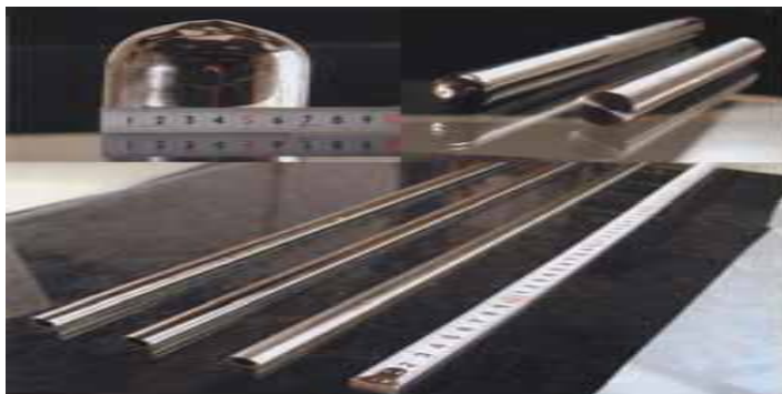
Fig. 1 Shape and outer surface appearance of some bulk glassy alloys in massive, cylindrical rod and tube forms produced by water quenching and copper mold casting.
