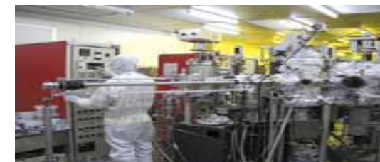
Molecular beam epitaxy (MBE)- sputtering equipment for the growth of III-V based ferromagnetic/nonmagnetic semiconductor heterostructures and magnetic metal devices.
