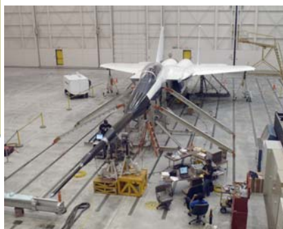
NASA Dryden Flight Research Center Photo Collection http://www.dfrc.nasa.gov/Gallery/Photo/index.html NASA Photo: E206-0254-115 Date: May 1, 2006 Photo By: Tony Landis NASA Dryden's F-15B aircraft with the Gulfstream Quiet Spike sonic boom mitigator attached undergoes ground vibration testing in preparation for test flights.
