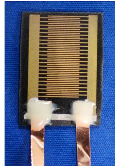
Rubber-based strain sensor fabricated using photolithographic lift-off process
