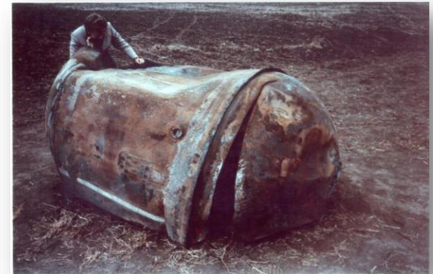
Fragment of a Delta second stage found in Texas on 22 Jan. 1997 (main propellant tank made of stainless steel, 250 kg)
