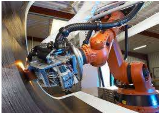
Automated Fiber Placement (Coriolis Composites)
