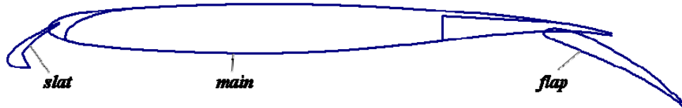
Fig. 1 Baseline airfoil and elements' settings.
