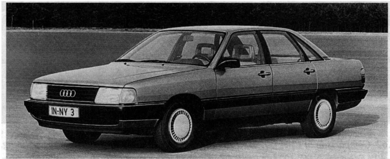
Fig. 1.63 The first car designed according to shape optimization, the Audi 100 III, 1978, c_D = 0.30 , A = 2.05 \text{ m}^2 .
