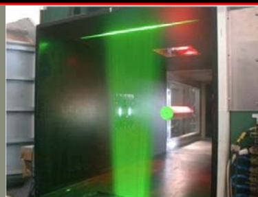
PIV Setup No. 2 (鉛直断面)
