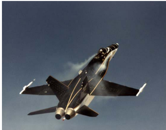
Dryden Flight Research Center EC89-0096-149 Photographed 1990 F-18 HARV flow-visualization smoke marks vortex flows along the leading edge extension. NASA photo
