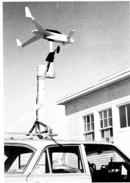
Fig. 2-4. Another view of car-top wind tunnel. (courtesy Burt Rutan)
