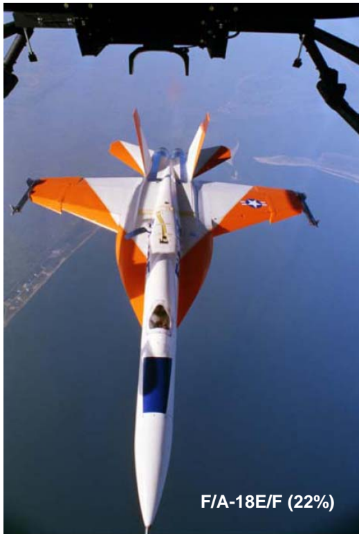
出典: Croom, et al "Research on the F/A-18E/F Using a 22 Percent Dynamically Scaled Drop Model", AIAA-2000-3913
