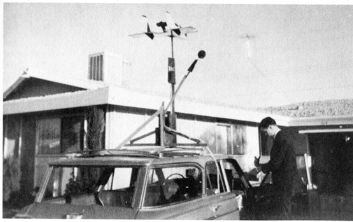
Fig. 2-3. Car-top wind tunnel mounted on 1966 Dart station wagon provided much early data that was not available from smaller school wind tunnels. Surprisingly, Rutan was never arrested for speeding during his 80-mph test runs. (courtesy Burt Rutan)
