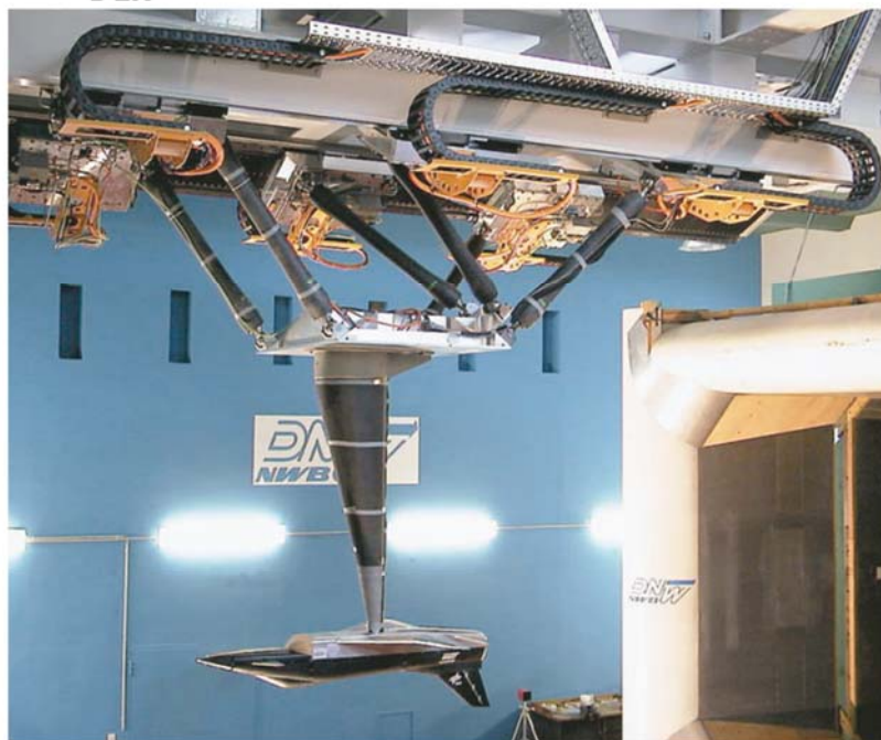
Figure 12: Fighter model suspended upside down from the MPM
