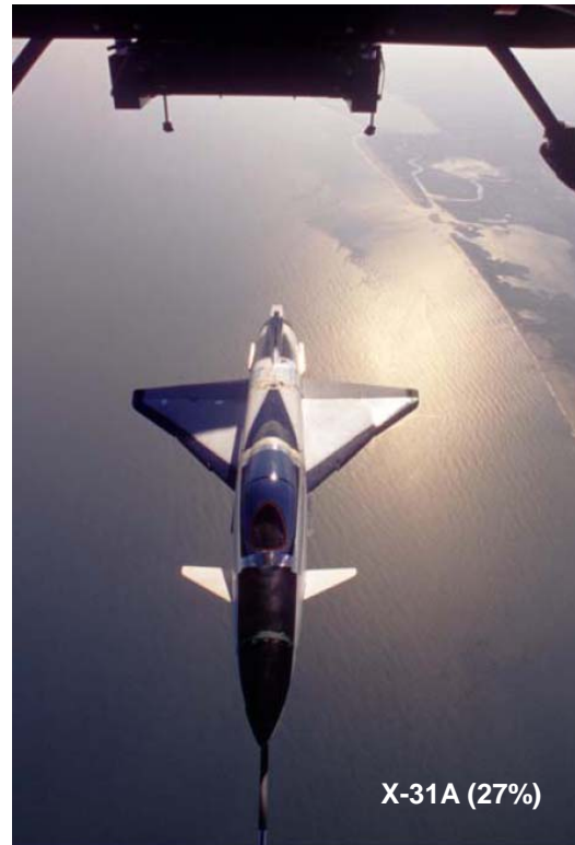
出典: Croom, Et al; "Dynamic Model Testing of the X-31 Configuration for High Angle-of-Attack Flight Dynamics Research", AIAA-1993-3674.
