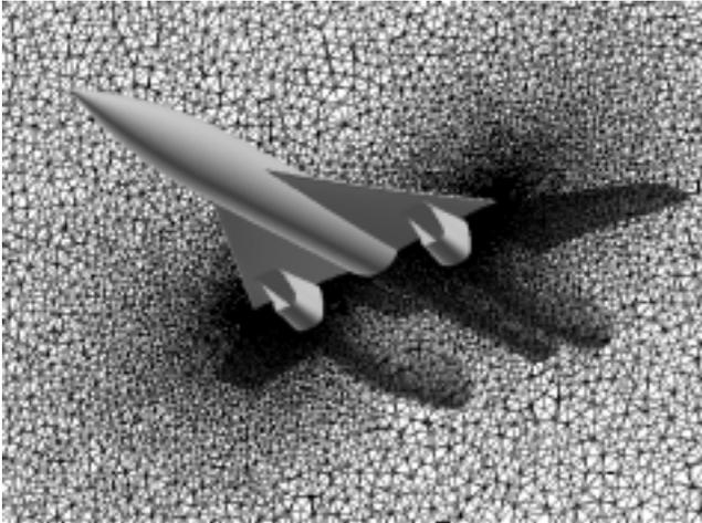
Fig. 6 Computational grid around a scaled supersonic airplane model
