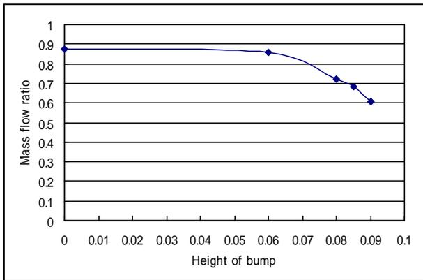
Fig. 4 Variation of mass flow ratios according to bump heights
