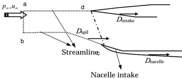
Fig. 5 Nacelle intake flow and streamlines
