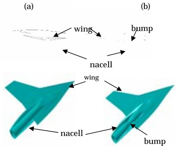
Fig. 3 Geometry of bump inside nacelle and cross sectional view of nacelle; (a) without bump, (b) with bump
