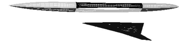
(d) Re-generated surface grid for wing and fuselage
