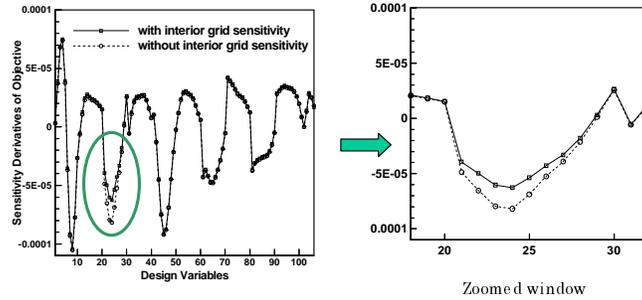
Fig. 1. Comparison of sensitivity derivatives with/without interior grid sensitivity
