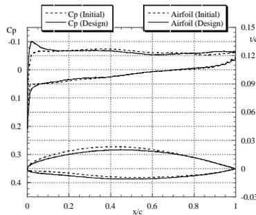
**Fig. 3.** Wing section shapes and pressure distributions for design example II ( $\eta = 0.3$ )
