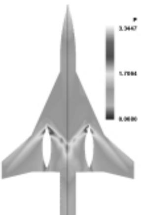
**Fig. 2.** Lower surface pressure contour of NAL experimental supersonic transport with nacelles, lower:initial, upper: design
