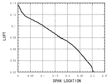
**Figure 4.** Loading distribution of the designed wing
