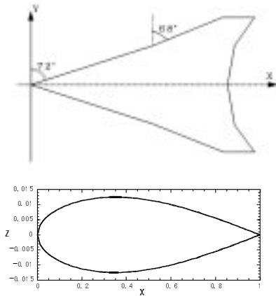
**Figure 1.** Wing planform and thickness distribution
