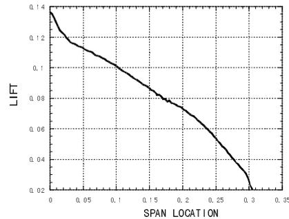
**Figure 4.** Loading distribution of the designed wing
