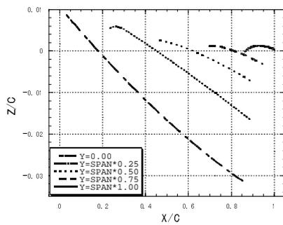
**Figure 5.** Camber lines of the designed wing
