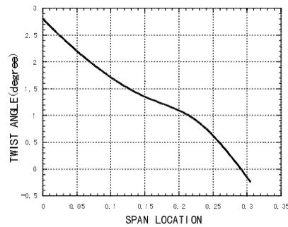
**Figure 3.** Twist angle distribution of the designed wing
