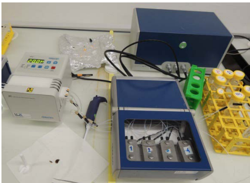
Quartz Crystal Microbalance (QCM)
