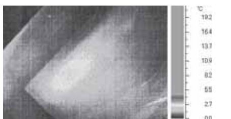
Fig.4 Surface temperature visualization by using infrared camera
