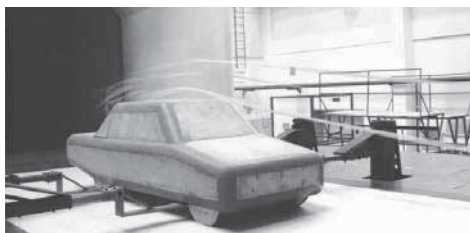
Figure 1: Experimental verification in Jilin University Wind Tunnel
