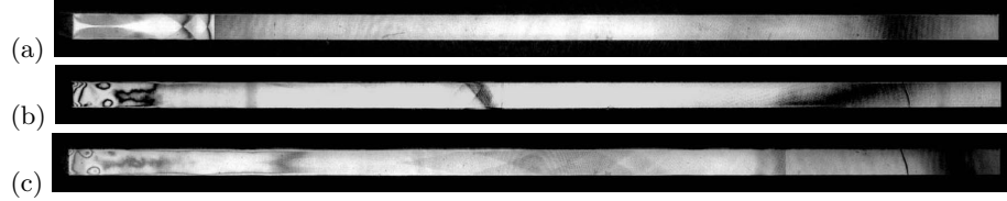
Fig. 4. Shock propagation in a channel, h = 8\text{mm} , p_0 = 10^5\text{Pa} , M_s = 1.2 : (a) t = 100\mu\text{s} ; t = 300\mu\text{s} ; t = 500\mu\text{s} .
