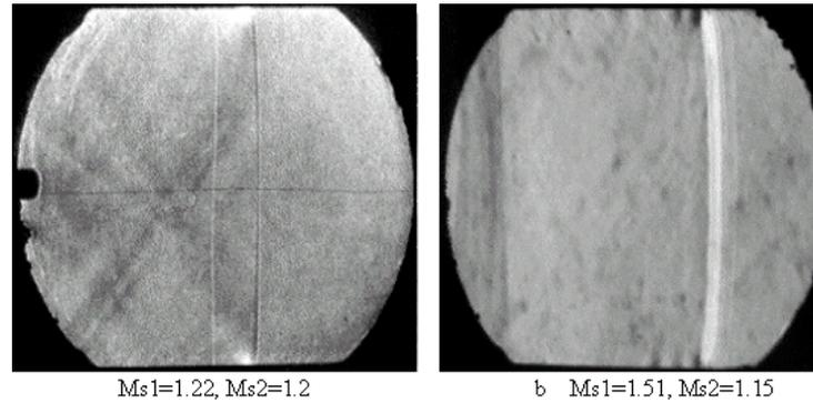
**Fig. 2.** Schlieren photos of down stream-facing shock wave/boundary layer interaction
