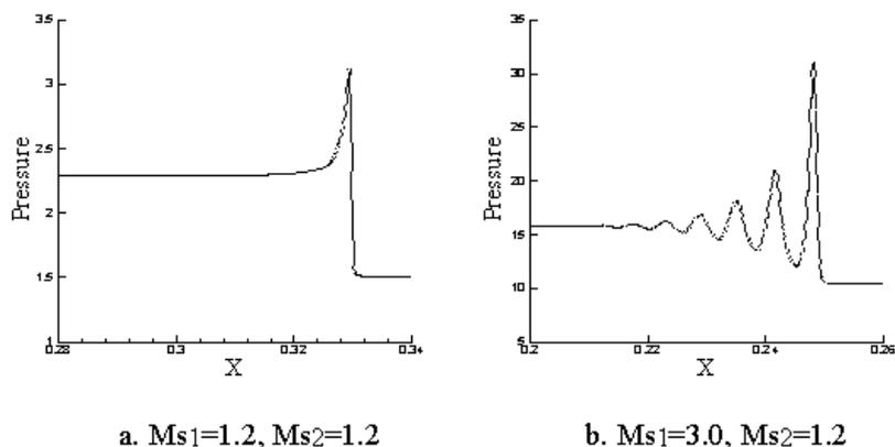
**Fig. 5.** Pressure distribution along the wall surface.
