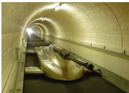
流動環境シミュレータ実験設備 Hyuga Aerodynamic Research by Towing (HART)
