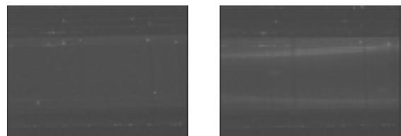
Fig. 3 Photographs indicating the occurrence of white turbidity at  $\dot{\gamma}^{(NW)} = 6.0\text{s}^{-1}$  (left) and  $41\text{s}^{-1}$  (right).
