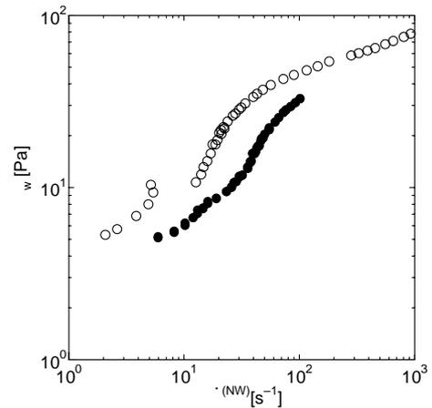
Fig. 1 Flow curves for a stainless steel capillary (open circles) and a glass capillary (filled circles)
