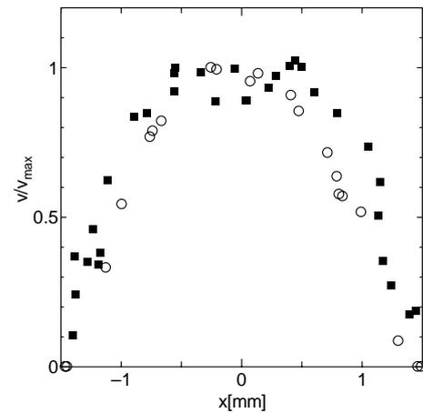
Fig. 2 Velocity profiles at  $\dot{\gamma}^{(NW)} = 6.0\text{s}^{-1}$  (open circles) and  $41\text{s}^{-1}$  (filled squares)
