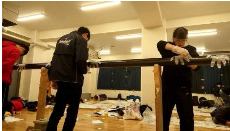
▲ CFRP Tube Production (Aug. ~ Dec. 2019) The airplane mainly consists of ~120 CFRP tubes. While some of HPA builders buy them from manufacturers, we make by ourselves.
