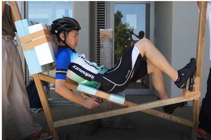
Frame Mock-up Fit Check (Sep. 2019) Confirmed that the frame fits for pilot's position and its design was appropriate.
