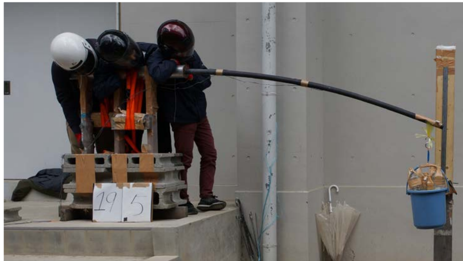
Material Strength Test (Sep. 2019) Acquired CFRP strength for safe structural design, also checked making procedure of spar.
