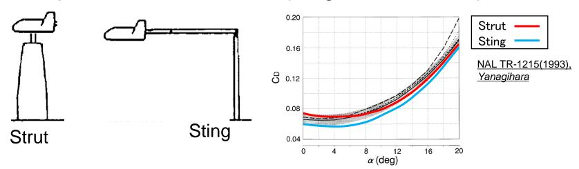
We need to conduct wind-tunnel tests without support
