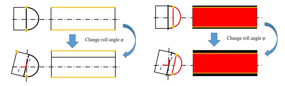
Color coding to two colors prevents interference of reflected light
