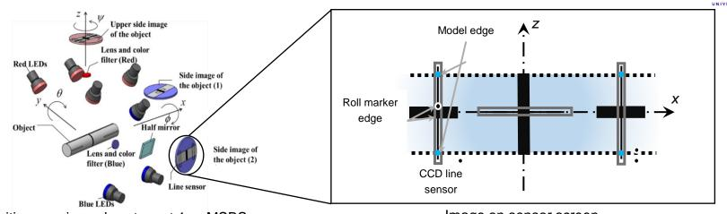
Position sensing subsystem at 1-m MSBS
