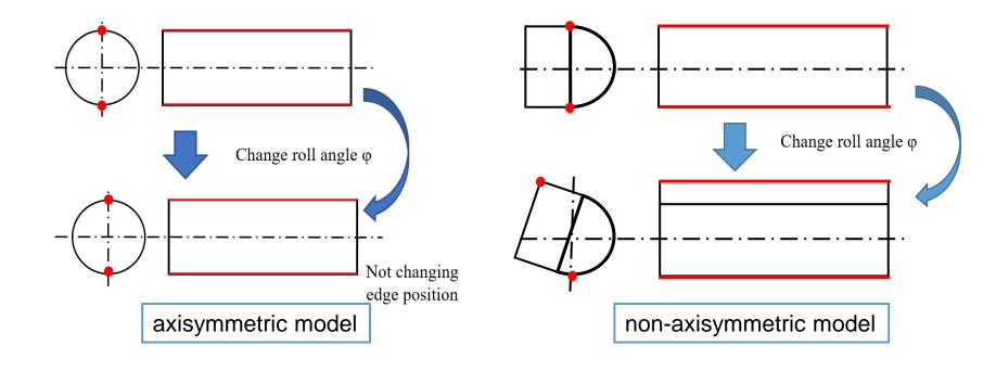
Non-axisymmetric model, the edge position changes when a roll angle occurs
