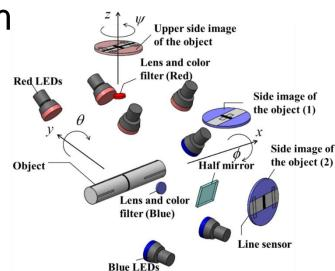
Position sensing subsystem at 1-m MSBS
