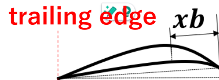
⇒ Max camber is at near trailing edge
