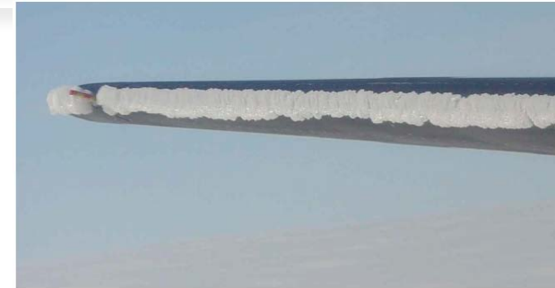
An example of icing at the leading edge of a main wing*
