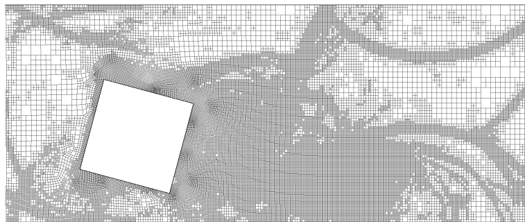
Figure 4.33. Shock / square-cylinder interaction, isopycnics and corresponding adaptive meshes (Continued). e.f. t = 2.0 , 38383 cells, CPU time = 82.0s; g.h. t = 3.0 , 48334 cells, CPU time = 147.6s, 1767 steps.
