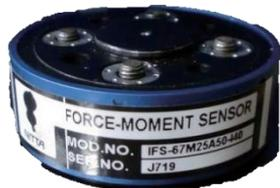
Force and Torque(F/T) Sensor
