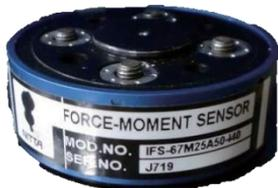
Measuring force and torque
