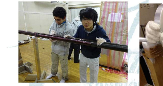
Lamination Ply1 90° Ply2 0° Ply5~ base on Ply3 45° each design Ply4 -45°
