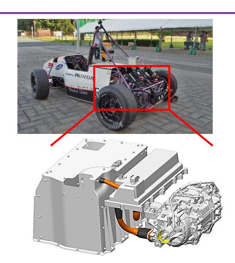
**Feature :** Battery, Inverter, Motor unit Supplied by Honda R&D Co., LTD.
