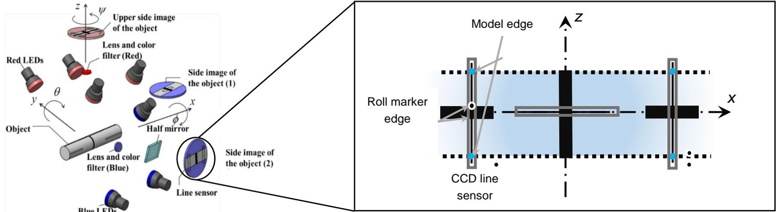
Position sensing subsystem at 1-m MSBS
