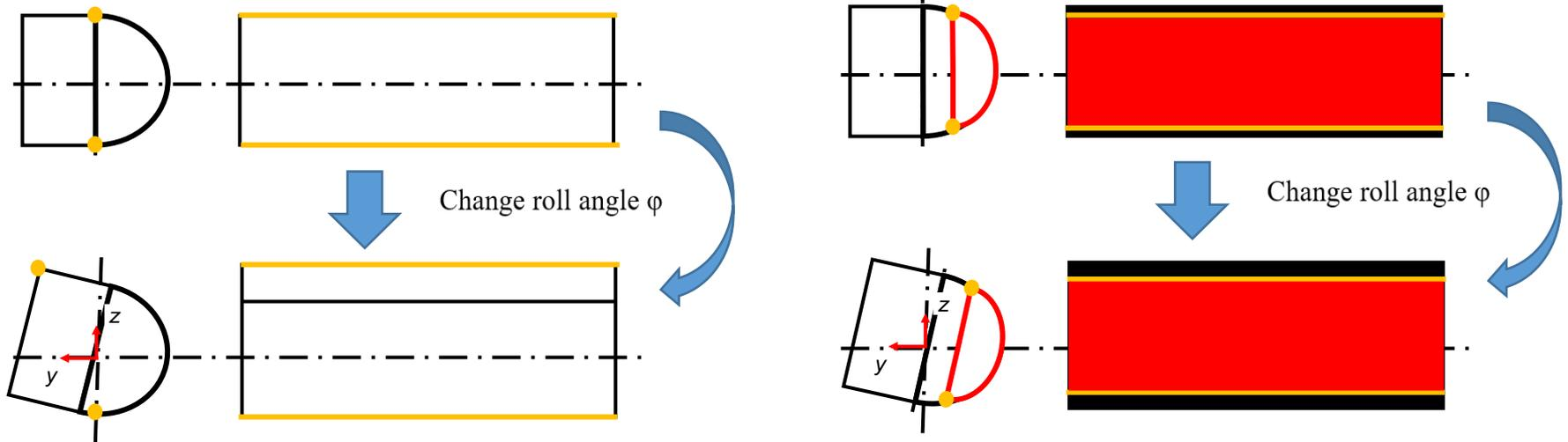
Color coding to two colors prevents interference of reflected light
