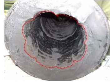
Fig. 8 The burned fuel surface just after mixing enhancer.
