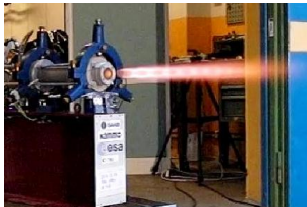
Fig. 3 \text{H}_2\text{O}_2 fed HRE during burn
