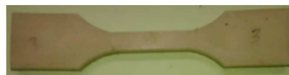
Fig. 3 Fuel specimen obtained by cooling at 313 K
