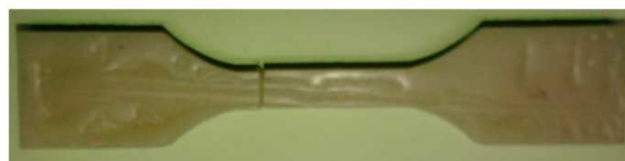
Fig. 2 Fuel specimen obtained by cooling at 300 K
