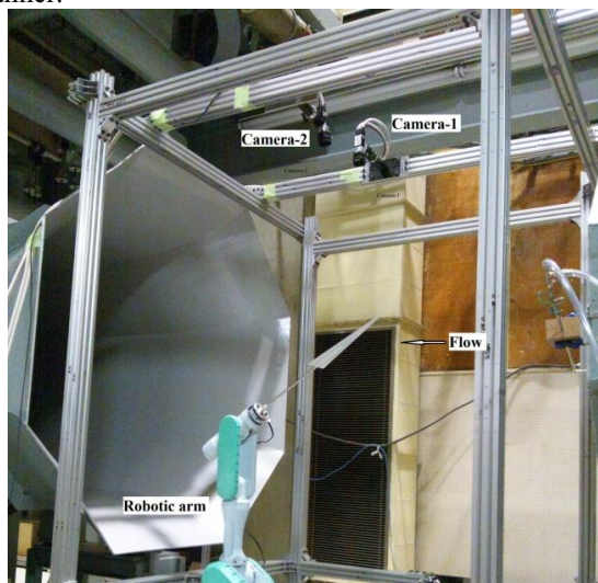
Fig. 1 Delta wing mounted using robotic arm
