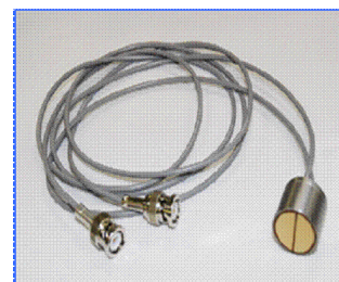
Fig. 2 Ultrasonic sensor with two cables, one is for pulsar and the other one is for receiver.
