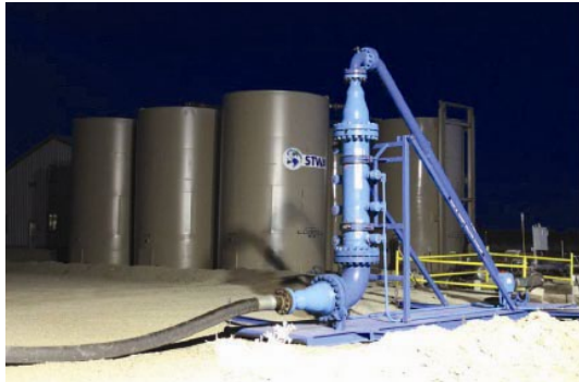
Fig. 5. The viscosity reduction device is connected in the pipeline.
