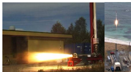
Fig. 2 Static firing and flight of a LOX fed staged-combustion HRE
