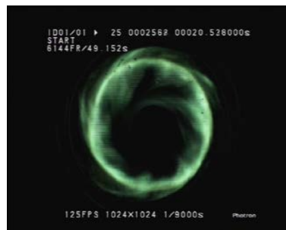
Figure 1 – Swirling injection of GOX in HTPB fuel grain.
