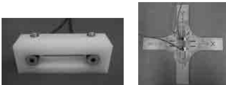
Figure 1: PECT probe (left) and biaxial test-piece of SUS316 stainless steel (right)
