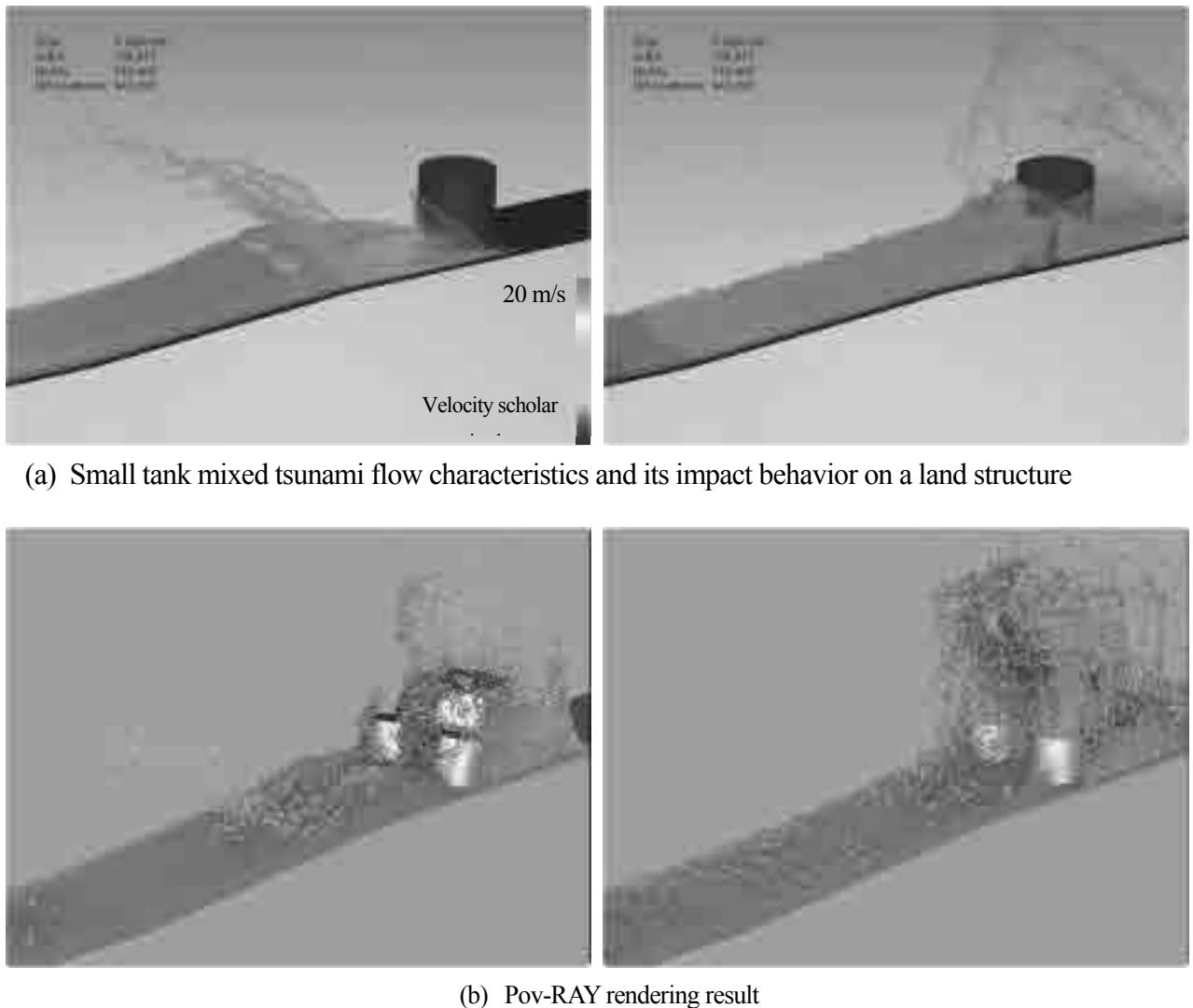
Fig. 7. Flotsam mixed tsunami flow characteristics and behavior of its interface deformation and collision with a land structure by SPH method.
