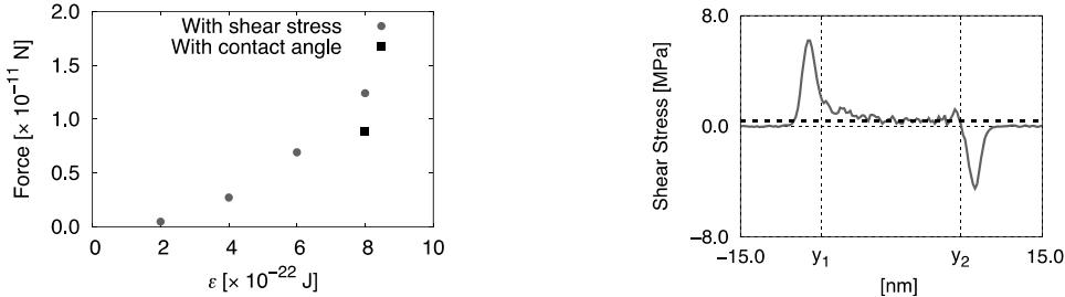
Figure 2 (a) Shear stress distribution in the case that  $\epsilon=8 \times 10^{-22}$  J. (b) Interaction parameter dependence of force on the interface. Red circles show the force evaluated with shear stress, and black squares show the force evaluated with contact angles.
