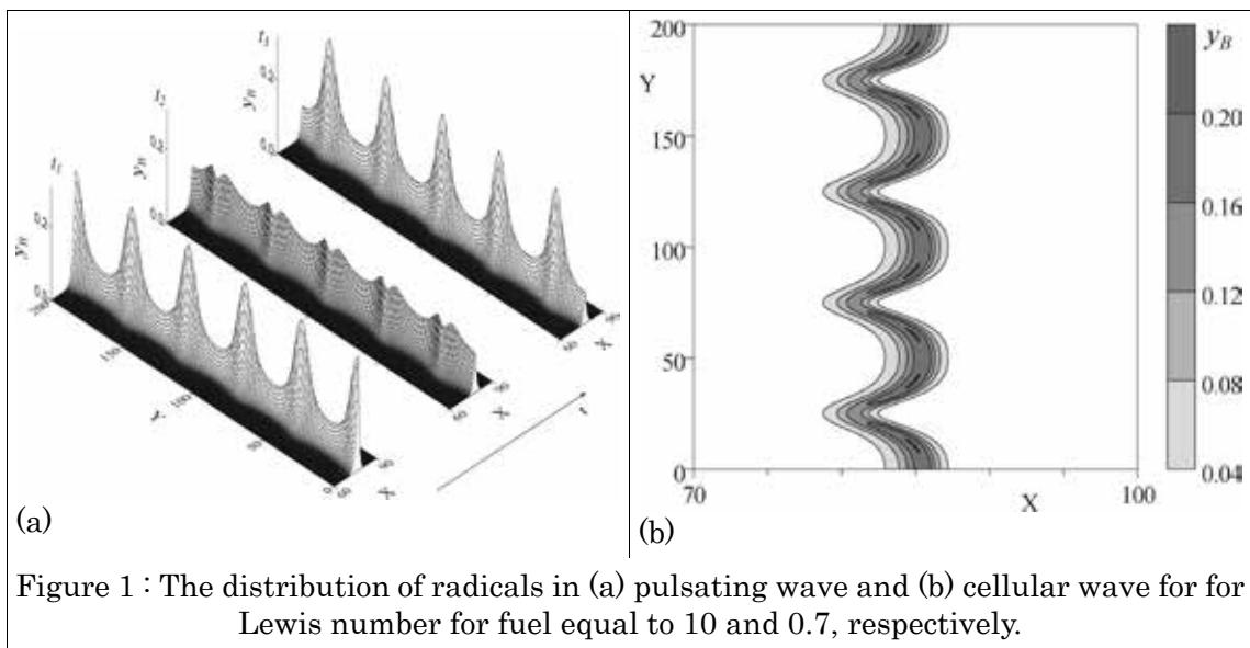
Figure 1 : The distribution of radicals in (a) pulsating wave and (b) cellular wave for for Lewis number for fuel equal to 10 and 0.7, respectively.
