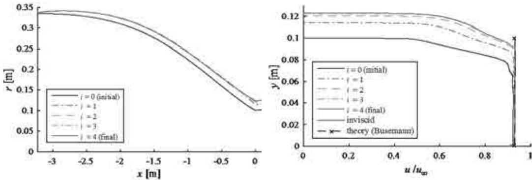
Figure 5 : Left: geometry progression (not to scale) in the viscous correction process starting with the inviscid geometry ( $i = 0$ ), right: progression of velocity profiles at the intake exit during the viscous correction iterative process for the full Busemann intake
