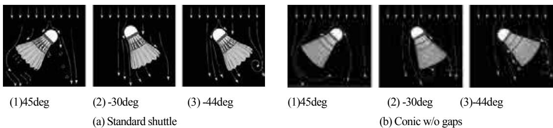
Fig.1 Schematic representation of flow field
