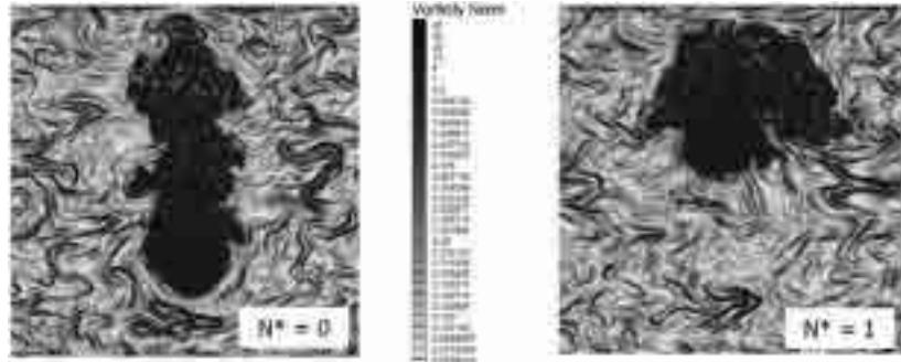
Figure 2 : Wake vortex comparison according to thermal stratification level at  $t^*=5$
