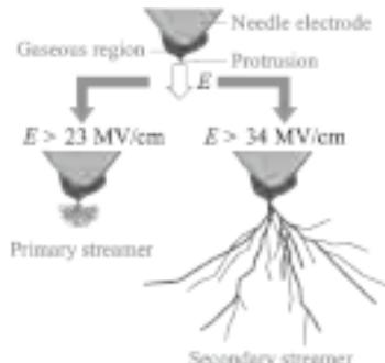
Fig. 2. Threshold electric fields for the inception of a primary streamer and a secondary streamer in water.
