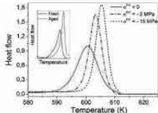
Figure 1: Effect of internal axial stress on the temperature dependence of heat flow.
