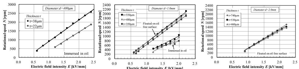
Fig.3 Effect of disk thickness  $t$
