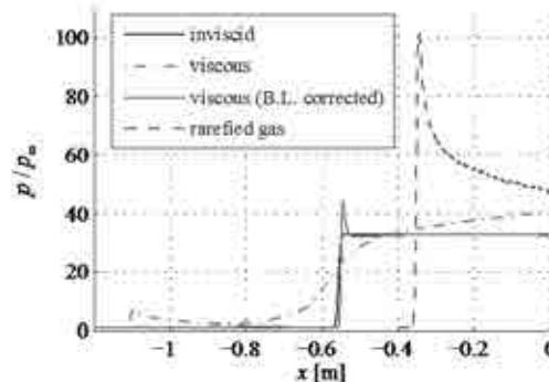
Figure 7 : Comparison of centerline pressure distributions for inviscid, viscous, and viscous-corrected flowfields in the continuum flow regime and that in the rarefied gas environment
