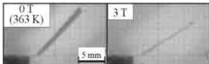
Fig. 4 Shape recovery process of the heat-treated Ni-Co-Mn-In film by applying the magnetic field.
