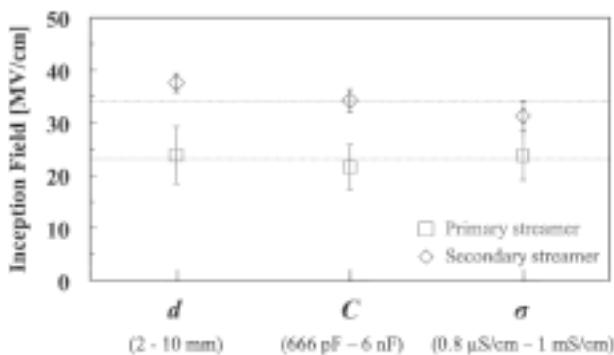
Fig. 1. Average inception fields acquired by changing the gap distance, the capacitance, and the water conductivity.
