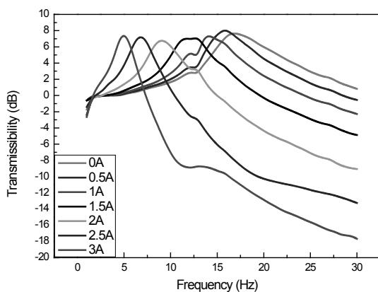
Figure 1: Transmissibility of the MRE isolator.
