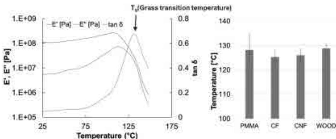
Figure 1: Dynamic moduli for PMMA and temperature of  $T_g$  with several composite materials
