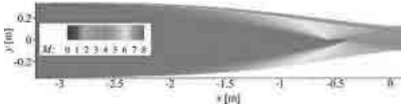
Figure 7 : Comparison of the Mach number distributions of the B.L.-corrected viscous (top) and rarefied gas ( $Kn = 0.003$ , bottom) flowfields for the full Busemann intake
