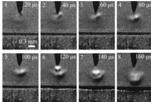
Figure: A series of Schlieren photos between the pin electrode and water surface. At 0 and 100-120  $\mu$ s, the plasma discharges were ignited.
