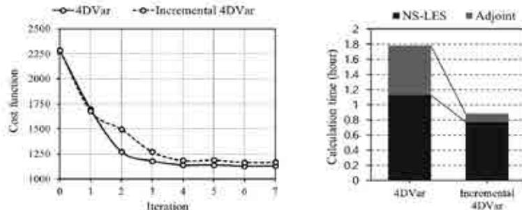
Figure 1: Cost function history and calculation time comparison.
