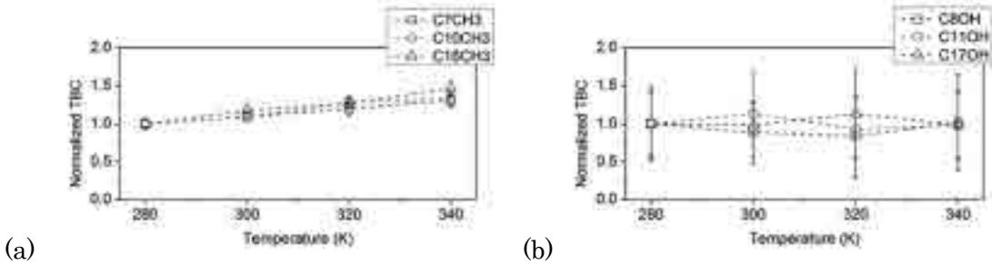
Figure 2: Normalized TBCs as a function of temperature. (a) CH<sub>3</sub>-terminated SAM; (b) OH-terminated SAM.
