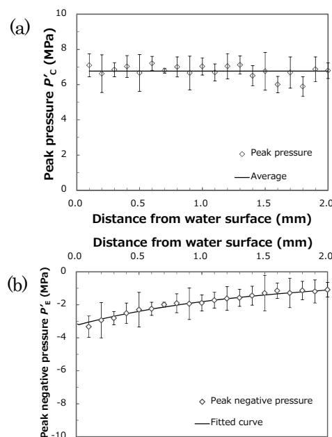
Fig. 1 (a) Peak pressure of the compressive wave against the distance from water surface and (b) peak pressure of the reflected expansion wave against the distance from the water surface.
