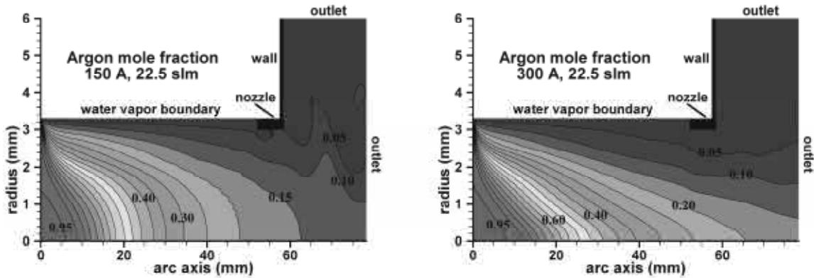
Figure 1. Isopleths of argon mole fraction for 150 A (left) and 300 A (right) discharges. Water mass flow rates are  $0.111 \text{ g} \cdot \text{s}^{-1}$  (150 A) and  $0.228 \text{ g} \cdot \text{s}^{-1}$  (300 A); argon mass flow rate is 22.5 slm for both currents. The increase of argon mole fraction in the centre of the arc for higher current is obvious. Contour increments are 0.05.
