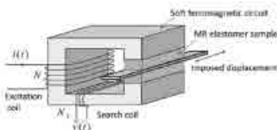
Figure 1 : Characterization bench for MRE properties measurements
