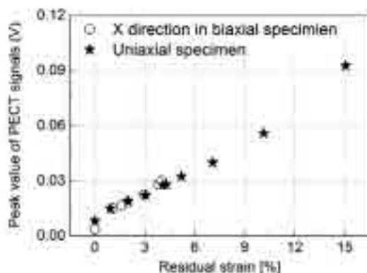
Figure 2: Comparison of peak signals for uniaxial and biaxial strain test-pieces
