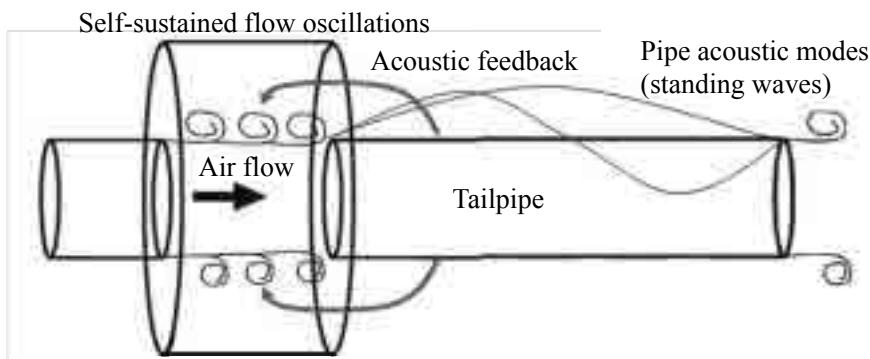
Fig. 1. Sketch of the cavity-tailpipe system. The black arrow indicates the direction of the flow. The red arrows symbolize acoustic feedback from the tailpipe to the self-sustained flow oscillations in the cavity.
