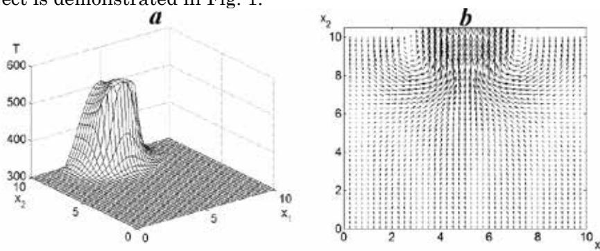
Figure 1: Example of the solid phase temperature (a) and the field of gas velocity (b) within the porous object.
