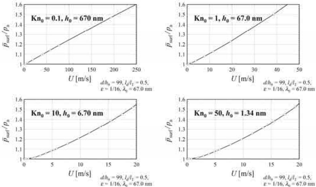
Fig. 2 Relation of the superficially averaged gas pressure  $\bar{p}_{\text{surf}}$  to the sliding speed  $U$ .
