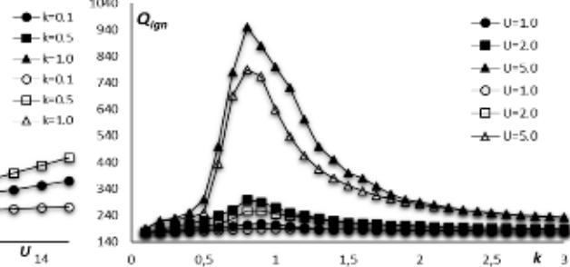
Fig. 2. Dependencies of minimum ignition energy on wave number
