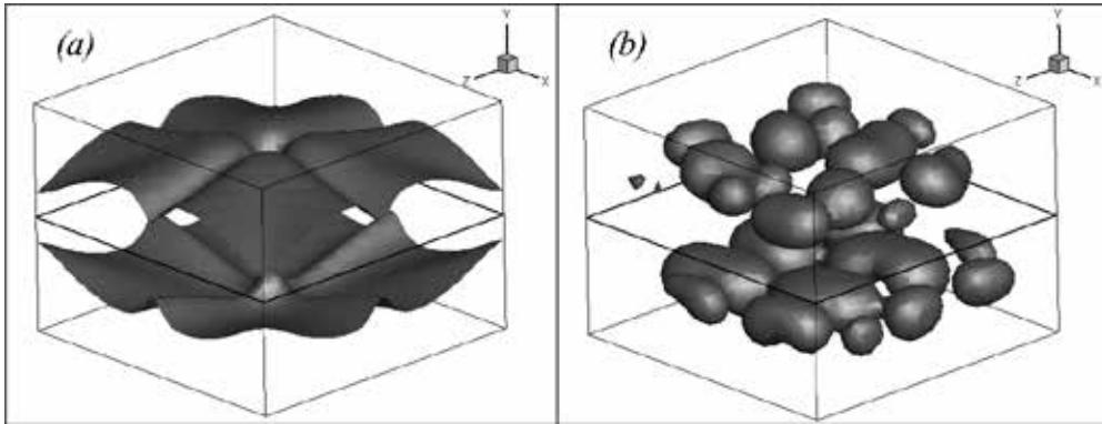
Figure1: Equiscalar surfaces of temperature that are typical for twin cellular flames (a) and sporadic combustion wave (b) in axisymmetric counterflow configuration.
