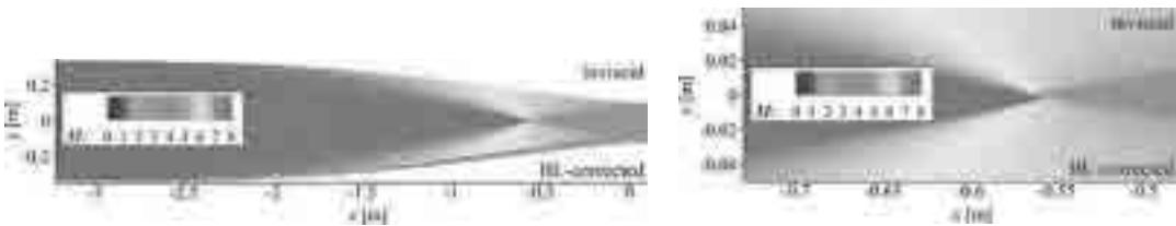
Figure 6 : Mach number distributions of the inviscid and viscous-corrected flowfields for the full Busemann intake (right: close-up)
