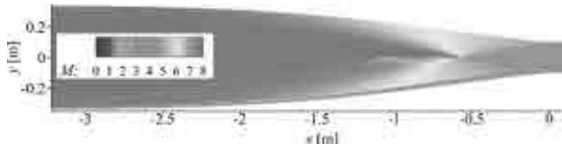
Figure 1 : Inviscid (top) and viscous (bottom) Busemann intake flowfields (Mach number)
