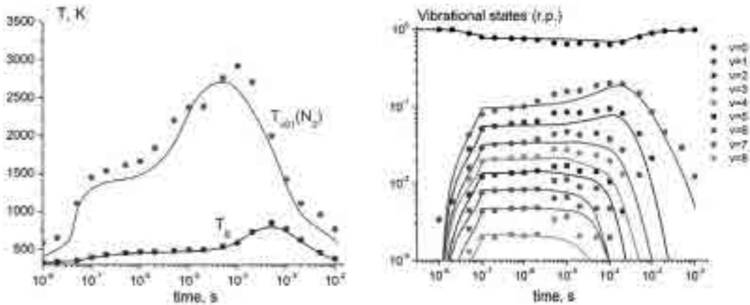
Figure 1. Left: Experimental and predicted time-resolved gas temperature and “first level”  $N_2$  vibrational temperature during and after the discharge pulse in air. Right: Experimental and predicted  $N_2(v=0-9)$  vibrational level populations, plotted vs. time after beginning of the main discharge pulse in air. Symbols: experimental data, lines: model predictions.
