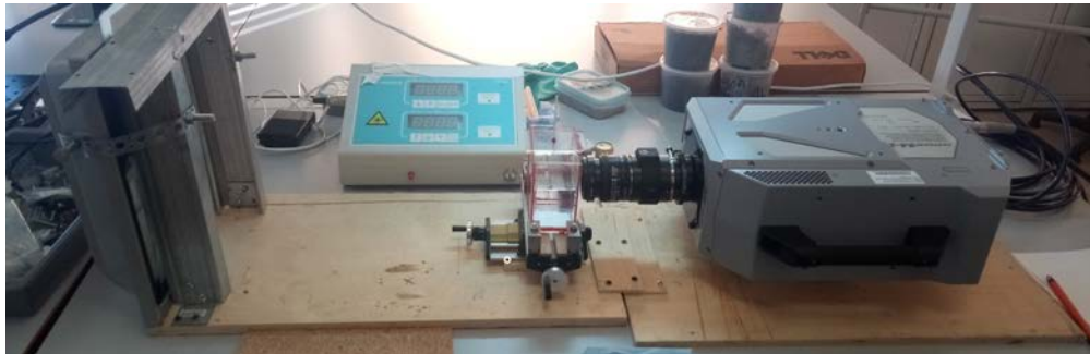
Fig. 6 Experimental system to observe bubble dynamics around the optical fiber
