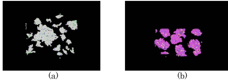
Figure 3 : The snapshot of (a) MXene-Fluid and (b) hBN-fluid at the same timestep. Mxene-fluid tend to form more clusters than hBN fluid
