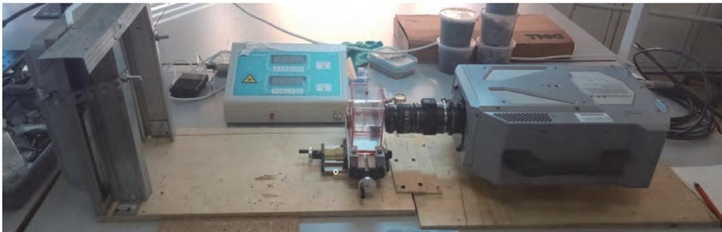
Figure 6: Experimental system to observe bubble dynamics around the optical fiber
