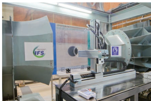
低乱熱伝達風洞の開放型測定部 Open test section of the low turbulence wind tunnel
