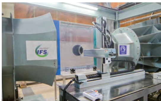
低乱熱伝達風洞の開放型測定部 Open test section of the low turbulence wind tunnel
